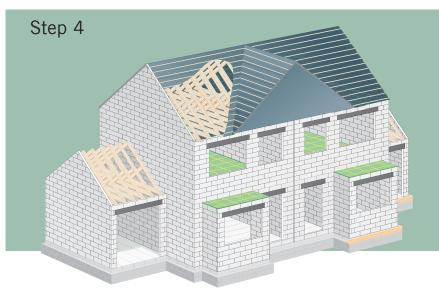
The build then continues apace with the second lift soon complete, with any gable ends built or spandrel panels positioned. The roof trusses are installed with felt and fly battens completing the Rå Build structure; handing the weather-tight masonry shell over to allow completion of the external leaf of the envelope whilst internally the first fix can start.
