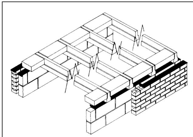
15.4 Normally, a whole block is used to bear on the first beam and the outside wall of a bay (except when a beam is laid alongside the wall). The block is bedded on the wall with a normal mortar joint. The unit compressive strength of the block must be equal to or greater than the unit compressive strength of the blocks used to form the wall. The mortar must be to the same specification as the mortar used for construction of the wall.
