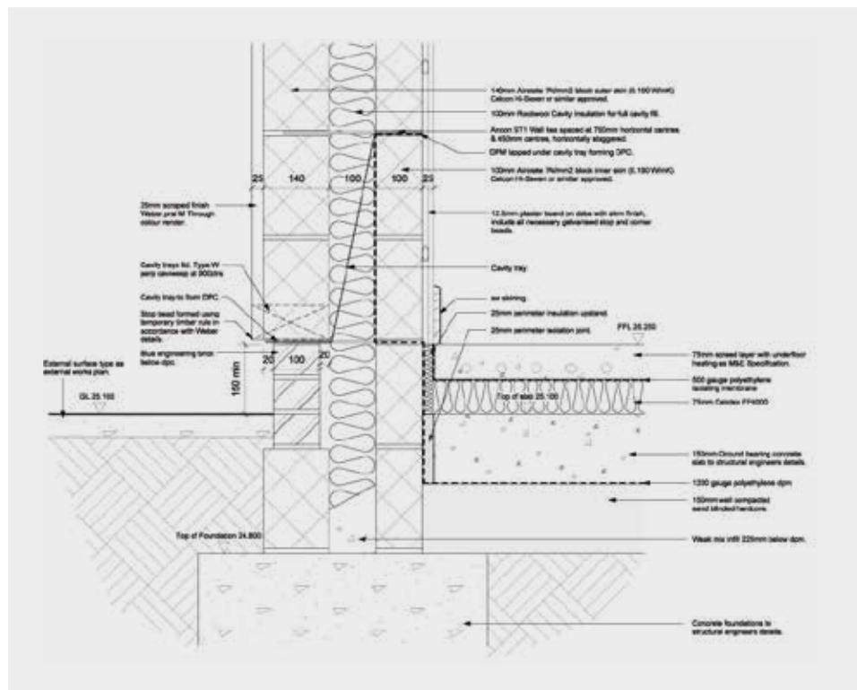
Weak mix infill, 225mm below dpm and then a further 150mm of well compacted sand blinded hardcore was applied directly above the concrete foundations.
