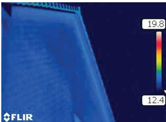
**Figure 11:** Thermal image of a gable end
